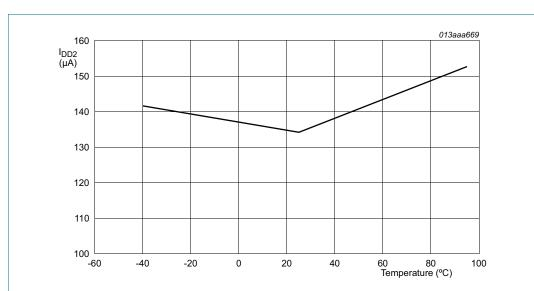
$V_{DD1} = V_{DD2} = 5.0 \text{ V}$ ; 1:4 multiplex drive mode;  ${}^{1}\!\!/_{4}$  bias; temperature measurement enabled; flat temperature compensation; LCD outputs are open circuit; RAM all logic 1; inputs at  $V_{SS}$  or  $V_{DD}$ ; internal clock with max prescale factor; bus inactive; charge pump on; charge pump configuration:  $V_{LCD} = 2 \times V_{DD2}$ ; VPR[7:0] set to 7.0 V; display enabled.
