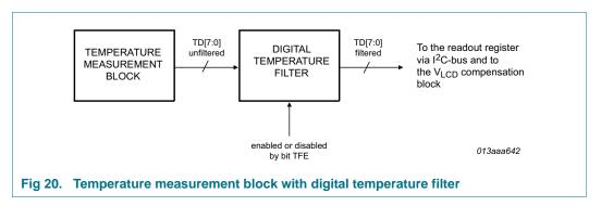
Like any other filtering, the digital temperature filter (see <u>Figure 20</u>) introduces a certain delay in the measurement of temperature. This behavior is illustrated in <u>Figure 21</u>.
