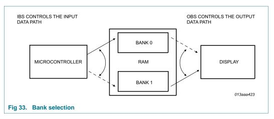
In <u>Figure 34</u> an example is shown for 1:4 multiplex drive mode where the displayed data is read from the first four rows of the memory (bank 0), while the transmitted data is stored in the second four rows of the memory (bank 1).
