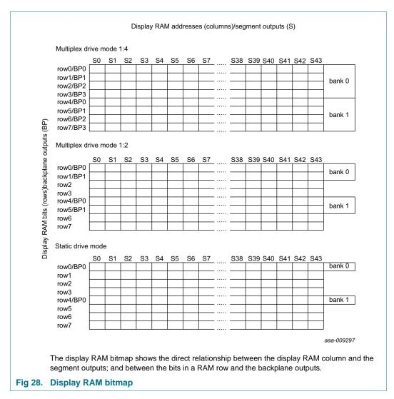
The display RAM bit map, <u>Figure 28</u>, shows row 0 to row 7 which correspond with the backplane outputs BP0 to BP3, and column 0 to column 43 which correspond with the segment outputs S0 to S43. The number of rows is twice the number of backplane outputs allowing to use two different RAM banks (see <u>Section 8.9</u>).
