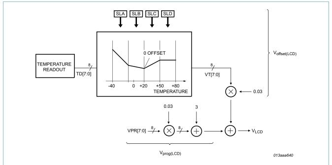
VPR[7:0] is the binary value of the programmed voltage. VT[7:0] is the binary value of the temperature compensated voltage. Its values come from the temperature compensation block and is a two's complement which has the value 0h at 20 °C.
