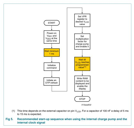
If the display is enabled too soon after the charge pump is enabled, then the  $V_{LCD}$  voltage may not have yet stabilized leading to an uneven display effect.
