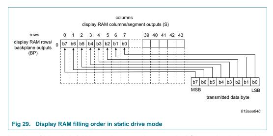
In order to fill the whole RAM row, 6 bytes must be sent to the PCA8547, but the last 4 bits from the last byte are discarded (see <u>Figure 30</u>).
