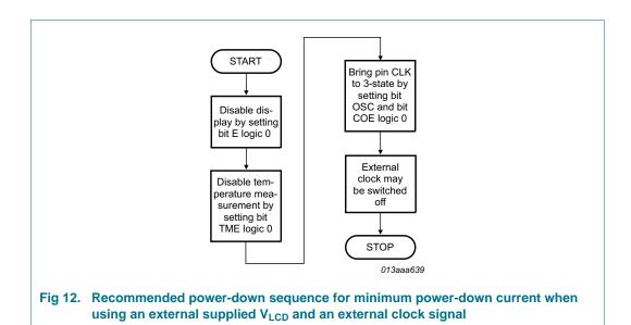
**Remark:** It is necessary to run the power-down sequence before removing the supplies. Depending on the application, care must be taken that no other signals are present at the chip input or output pins when removing the supplies (see <u>Section 10</u>). Otherwise this may cause unwanted display artifacts. In the case of uncontrolled removal of supply voltages the PCA8547 will not be damaged.
