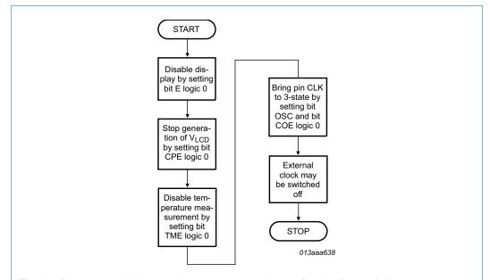
Fig 11. Recommended power-down sequence when using the internal charge pump and an external clock signal
