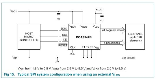
The host microcontroller maintains the two-line  $I^2C$ -bus communication channel with the PCA8547A or the three-line SPI-bus with the PCA8547B. The appropriate biasing voltages for the multiplexed LCD waveforms are generated internally. The only other connections required to complete the system are the power supplies ( $V_{DD1}$ ,  $V_{DD2}$ ,  $V_{SS}$ ,  $V_{LCD}$ ), the external capacitors, and the LCD panel selected for the application.
