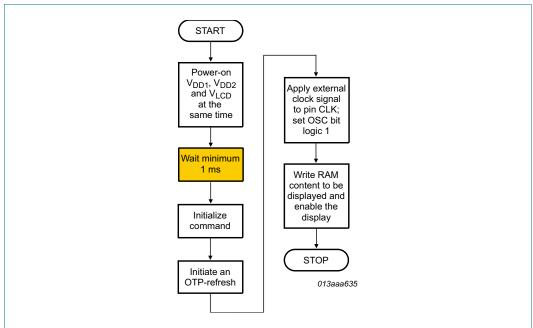
Fig 8. Recommended start-up sequence when using an external supplied  $V_{\text{LCD}}$  and an external clock signal
