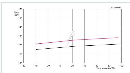
$V_{DD2}$  = 5.0 V; 1:4 multiplex drive mode;  $\mathcal{V}_4$  bias; temperature measurement enabled; LCD outputs are open circuit; RAM all logic 1; inputs at  $V_{SS}$  or  $V_{DD}$ ; internal clock with max prescale factor; bus active.
