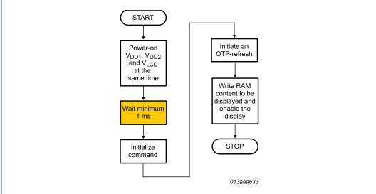
Fig 6. Recommended start-up sequence when using an external supplied  $V_{\text{LCD}}$  and the internal clock signal
