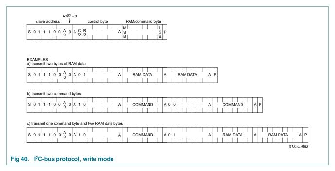
The display bytes are stored in the display RAM at the address specified by the data pointer.
