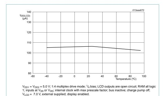
Fig 51. Typical  $I_{DD(LCD)}$  with respect to temperature
