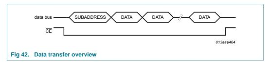
The subaddress byte opens the communication with a read/write bit and a subaddress. The subaddress is used to identify multiple devices on one SPI-bus.
