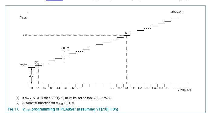
Figure 17 illustrates how V<sub>LCD</sub> changes with the programmed value of VPR[7:0].
