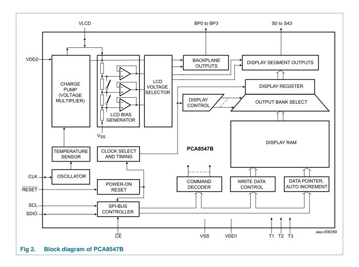
x 44 automotive LCD driver with integrated charge pump
